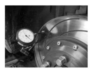
The tolerance of oscillate value of rotor moving up and down cannot exceed 0.15mm.
