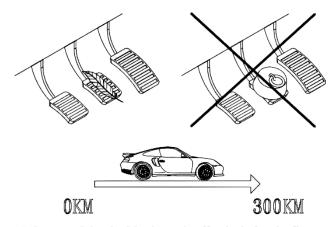
It is essential to bed-in the pads effectively for the first 0-300km to protect the brake disc from being deformed.
