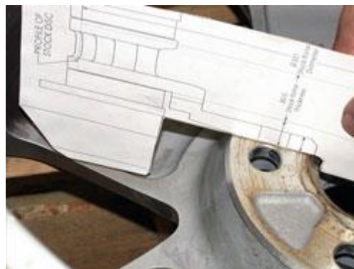
4. Verify that edge of the caliper does not touch the rim or the spoke. A minimum of 2mm (0.080") is recommended.
