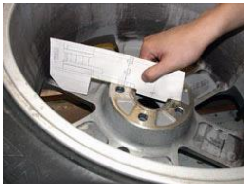
3. Lay the template inside the wheel as shown
